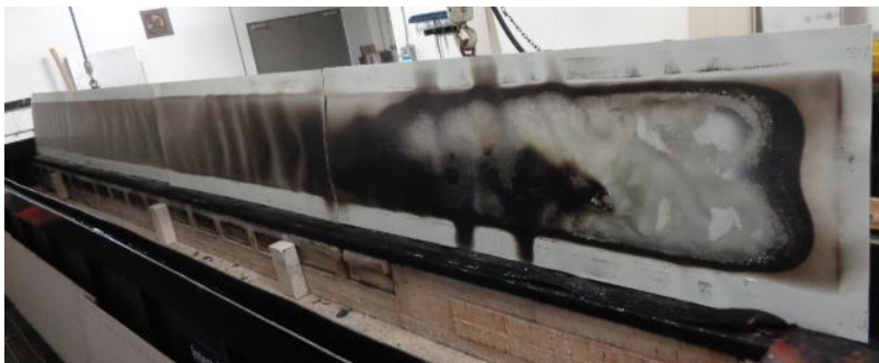
Photo No. 4 Exposed Surface of the Test Specimen (Post-test)
