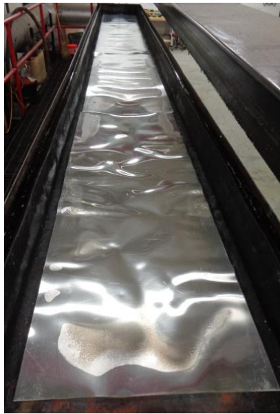
Photo No. 3 Unexposed Surface of the Test Specimen (Post-test)
