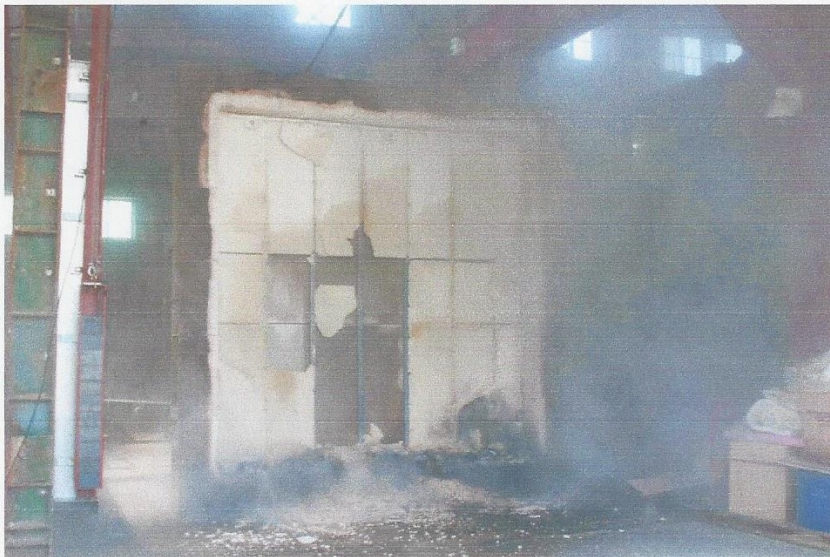
Exposed face of the specimen after hose stream test
